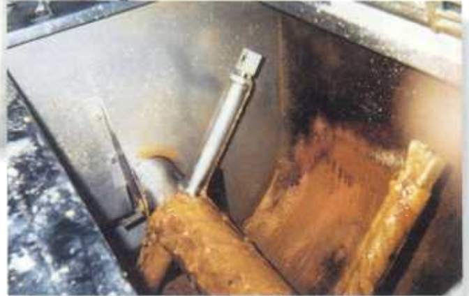
Figure 3: Partially cleaned mixer in a sweets factory
